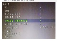
**CONTRAST:** By setting "MANUAL" it is possible to manually modify the contrast values, from 0 to 20 (default 7). In this case the camera will respect the set value.
