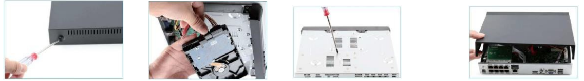
1. Remove the case 2. Connect the SATA cable 3. Screw the HDD all the way in 4. Install the case
